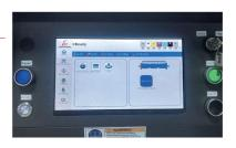
The simple and intuitive 10" Color LCD Touch Screen provides loading & unloading control, printhead maintenance, and real-time printing parameter settings.
